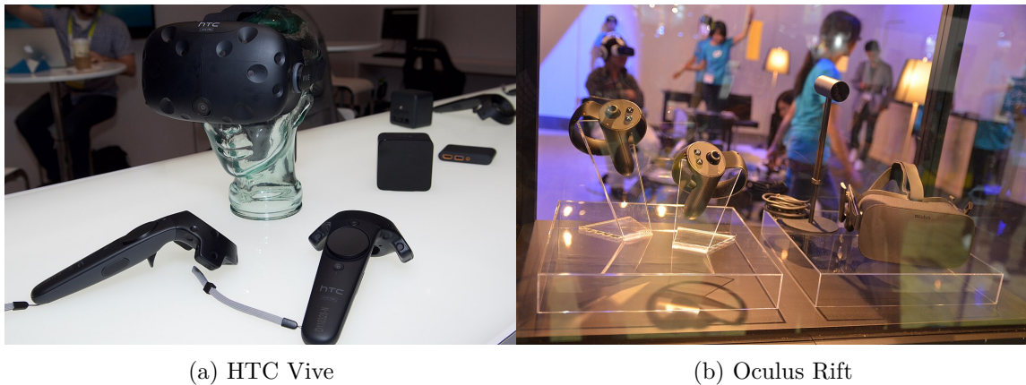
Figure 2.2: The first consumer oriented VR headsets, from 2016, HTC Vive and Oculus Rift.
